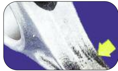
Figure 1 - No Core Refund Crank bore is scored and heat discoloured
