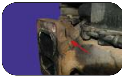
Figure 2 - Full Core Refund Operational damage - crack
