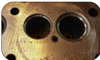
Figure 4 - Damaged Core Refund Dropped valve damage
