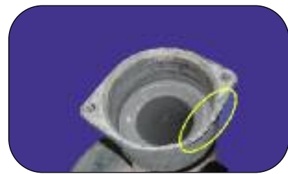
Figure 3 - Full Core Refund Damage - chipped cold housing
