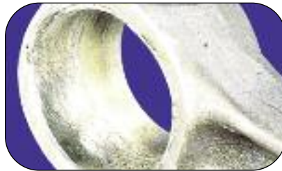
Figure 3 - No Core Refund Pin bore damage
