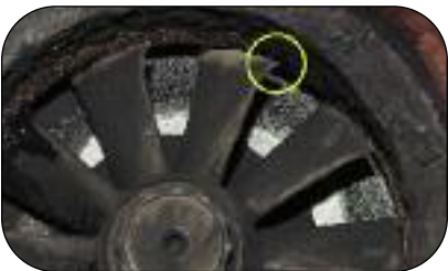
Figure 6 - Damaged Core Refund Hot wheel bent
