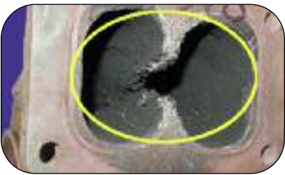
Figure 4 - Full Core Refund Webbing burned out
