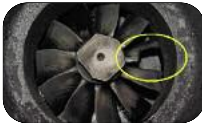
Figure 7 - Damaged Core Refund Hot wheel broken
