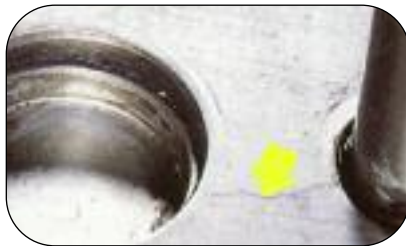
Figure 3 - Damaged Core Refund Top deck crack
