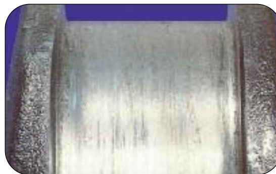
Figure 6 - Full Core Refund Bearing build-up
