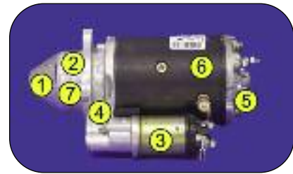
Figure 1 - Typical Illustration of Starter Subassemblies
